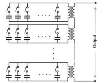
With  $n$  capacitors,  $m$  modules, capacitor voltage rating of  $V$ , and capacitor current rating of  $I$ , the output pulse has current= $nI$  and peak voltage= $mV$ .
