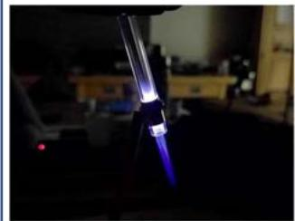
You can see the pin electrode on the inside of the glass and the ring electrode is the dark part on the outside of the glass.
