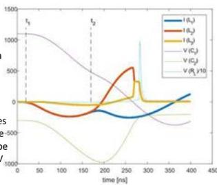
The graph depicts a simulation of a circuit that uses inductor(L) and capacitor(C) pairs coupled with the DSRD to form pulses. The increase in voltage can be seen as the peak voltage over the capacitor is -1kV and the peak output voltage (RL) is 10kV.
